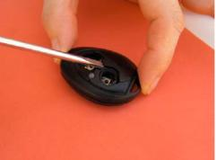
With flat small screw-driver "shave off" top layer. Do not pull rubber, to avoid breaking shell and exposing small holes in the surface
