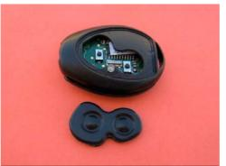
Button replacement silicone pad has to be press fitted over the cut out
