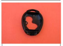
All soft layers have been removed to expose entire cut out in hard plastic part
