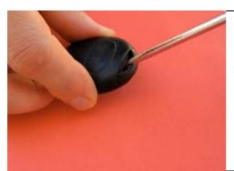
☐ Use small flat screw-driver to open remote key on the split line and to separate it into two parts
