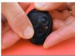
Place Silicone pad over cut out and push it in, so it "engages" with plastic cover
