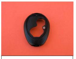
Hard plastic part is ready for fitting of new silicone replacement pad
